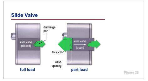
At full load, the slide valve is closed. The compressor pumps its maximum volume of refrigerant, discharging it through the discharge port.
